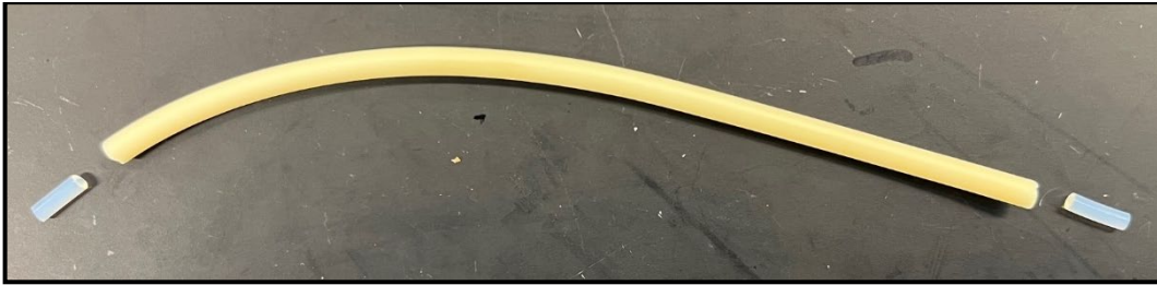
Figure 9: PTFE plugs (0.7 cm) to be inserted into both ends of the small-bore latex tubing (13 cm).
