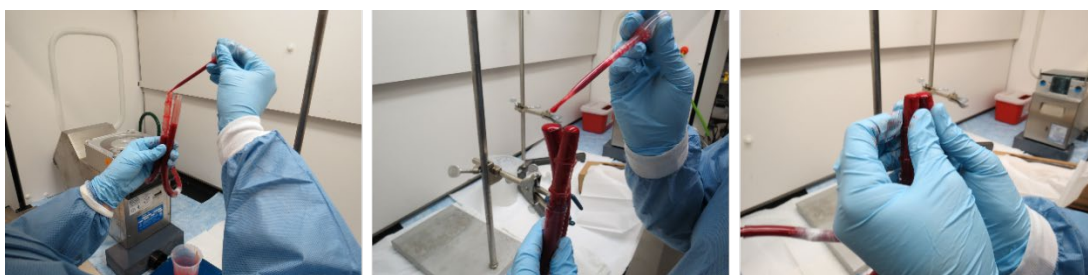
Figure 15: Images showing how to use a transfer pipet to completely fill the loop and remove bubbles
