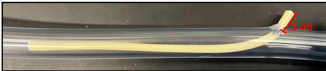
Figure 12: Side view of the latex tubing (plugged) inserted into the PVC tubing with 1 cm remaining outside (red).
