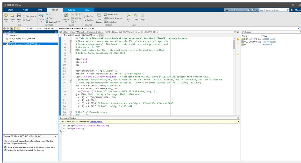
Results, including battery terminal voltage, depth of discharge (DOD), surface temperature, discharge current, and OCV-DOD characteristic curve, are plotted and stored in the MATLAB file directory.
