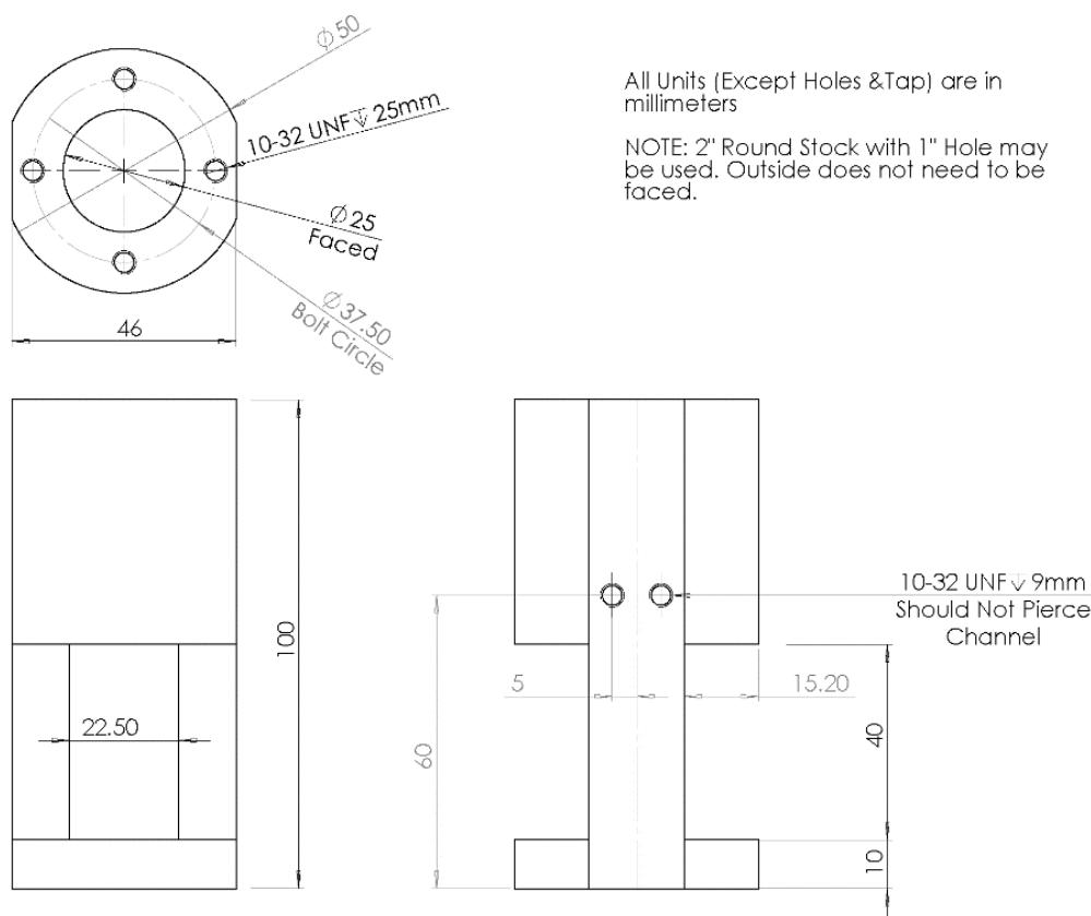
Figure 2: CAD Drawing of the Puncture Rig Setup Base
