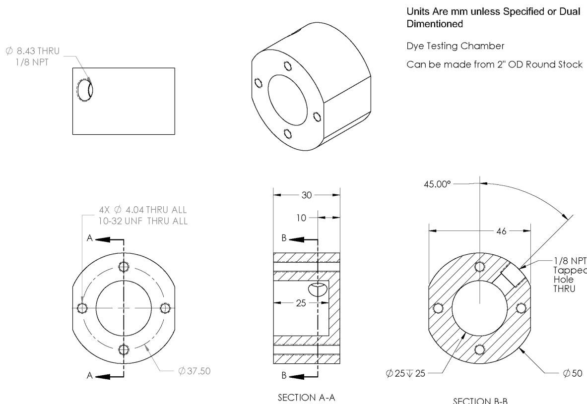
Figure 3: CAD Drawing of the Modified Dye Testing Cell to be Used in the Partial Puncture and Dye Testing.
