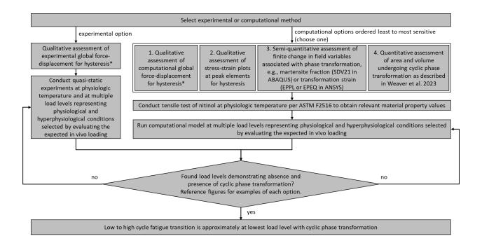
Figure 1: Flowchart to estimate low to high cycle fatigue transition.
