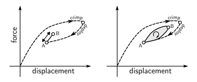
Figure 2: Experimental Option and Computational Option 1: Examples illustrating absence (left) or presence (right) of hysteresis when cycling between two loading points A and B.
